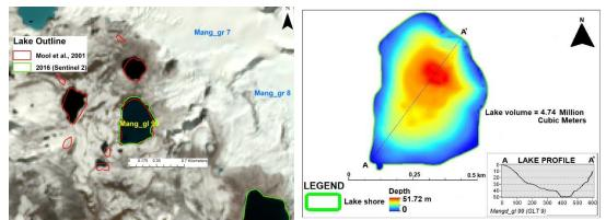
*Figure 3.16: Left:* Mang\_gl 99 with feeding glacier Mang\_gr 7. Green and red polygons are the lake outline from Sentinel 2 (2016) and Mool et al., 2001. *Right:* Lake bathymetry map of Mang\_gl 99 along with the lake depth profile from outlet to upper reach (A-A')
