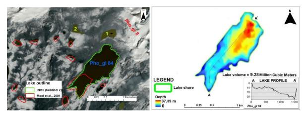
*Figure 3.6 :Left:* Pho\_gl 84 on Sentinel 2 (2016) with other adjacent lakes and feeding glacier Pho\_gr 8. Green and red polygons are the lake outline from Sentinel 2 and by Mool et al., 2001. Number 1 and 2 are the new lakes formed. *Right:* Bathymetry map of the lake with the depth profile A-A'
