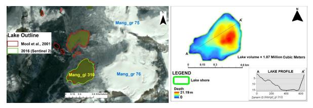
*Figure 3.22: Left:* Mang\_gl 310 (Zanam G) on Sentinel 2 (2016) imagery. The red polygon is the lake outline by Mool et al., 2001 and green is from Sentinel 2 (2016). *Right:* Bathymetry map of Mang\_gl 310 along with depth profile from outlet to upper reach (A-A').
