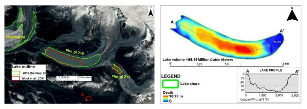
*Figure 3.13: Left:* Mo\_gl 210 (Lugge Tsho) on Sentinel 2 image. Green and red polygon are the Lake Outline from Sentinel 2 (2016) and Mool et al., 2001. Pho\_gl 211 is Drukchung lake. *Right:* Bathymetry map of Lugge lake (data from 2011). Due to lack of data coverage towards the upper reach, the depth interpolated is lesser.
