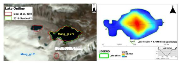
*Figure 3.19: Left:* Mang\_gl 207 (lake Zanam F) on Sentinel 2 (2016) image with lake polygons of Mool et al., 2016 (red) and Sentinel 2 (2016). *Right:* Lake bathymetry map with depth profile (A-A').
