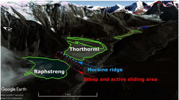
Figure 3.11: Raphstreng and Thorthormi lakes showing the location of thin and active moraine barrier
