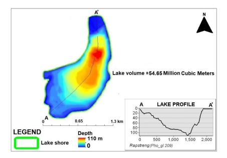
Figure 3.12: Bathymetry map of Raphstreng lake along with the depth profile (A-A')
