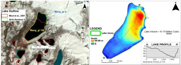
*Figure 3.17: Left:* Mang\_gl 106 (Metatshota) delineated using Sentinel 2 of 2016 (Green) IRS 1D of 1999 (Mool et al., 2001). *Right:* Lake bathymetry map prepared using the data set of 2009 (DGM-JICA/JST GLOF Project) along with depth profile A-A'
