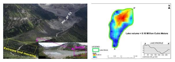
*Figure 3.4: Left:* Photo of Latshokarp show the location of Mo\_gr 51. The lake has a wide open outlet which is shown in pink rectangular box. Yellow dotted box shows the extreme end moraine. *Left:* Bathymetry map of the lake with the depth profiles A-A'.
