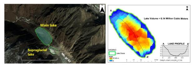
*Figure 3.5: Left:* Sintaphu glacial lake and the supraglacial lake on google earth pro image (imagery date: 1-4-2014). The lake boundaries are from the Sentinel 2 image (2016). *Right:* Bathymetry map of the main lake with depth profile from outlet towards upper reach (A'-A)
