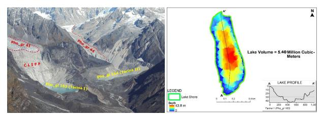
*Figure 3.8: Left:* Photo showing Tarina I, Tarina II, Pho\_gr 41, Pho\_gr 44 and the Cliff along which the Pho\_gr 41 feeds Tarina I in the form of ice fall. *Right:* Bathymetry map of Tarina I along with the depth profile from the outlet towards upper reach of the lake (A-A')
