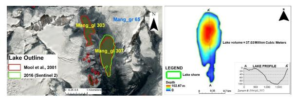
*Figure 3.21: Left:* Mang\_gl 307 (Zanam B) and Mang\_gl 303 (Zanam A) on Sentinel 2 (2016) imagery. The red polygon is the lake outlines by Mool et al., 2001 and green is from Sentinel 2 (2016). *Right:* Bathymetry map of Mang\_gl 307 along with depth profile from outlet to upper reach (A-A').
