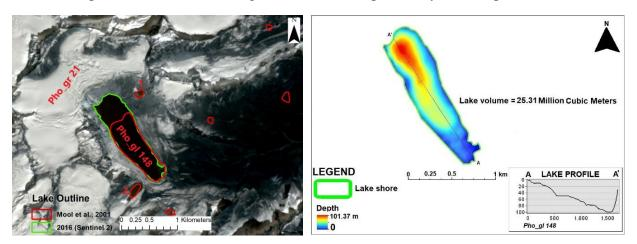
**Figure 3.7: Left:** Pho\_gl 148 with adjacent lakes lying at higher elevation (1&2) and the feeding glacier Pho\_gr 21 which wastes part of it in the form of icefall into the lake. Green and the red polygon shows the lake outline of 2016 (Sentinel 2) and Mool et al., 2001 respectively. Background image is Sentinel 2 (2016). **Right:** Bathymetry map of the lake with depth profile (A-*A*'). Lake has shallow depth at the outlet part and deeper towards the upper reach.
