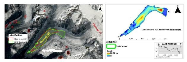
*Figure 3.27: Left:* Cham\_gl 383 (Chubda Tsho) on Sentinel 2 (2016) imagery. The red polygon is the lake outline by Mool et al., 2001 and green is from Sentinel 2 (2016). *Right:* Bathymetry map of Cham\_gl 383 along with depth profile from outlet to upper reach (A-A')
