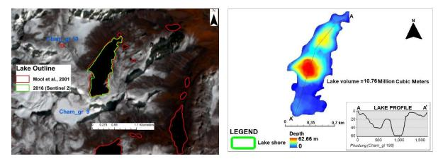
*Figure 3.24: Left:* Cham\_gl 198 (Phudung Tsho) on Sentinel 2 (2016) imagery. The red polygon is the lake outline by Mool et al., 2001 and green is from Sentinel 2 (2016). *Right:* Bathymetry map of Cham\_gl 198 along with depth profile from outlet to upper reach (A-A')
